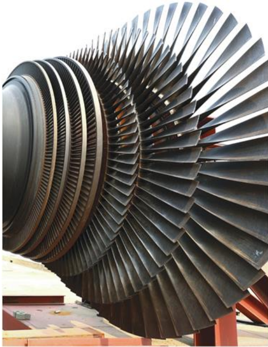
Turbine blades attached to the turbine shaft.
